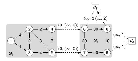
We will will use the routing and mapping of  $G_2$  to construct a forwarding  $\mathbf{F}_2$ , that will be passed as a mapping to  $G_1$  ...
