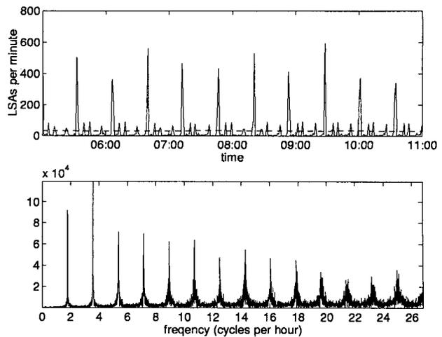
Fig. 7. Refresh-LSA traffic for routers running IOS 12. The upper graph shows the time-series for a few hours of a typical day. The lower graph shows the power-spectrum analysis of the time-series.
