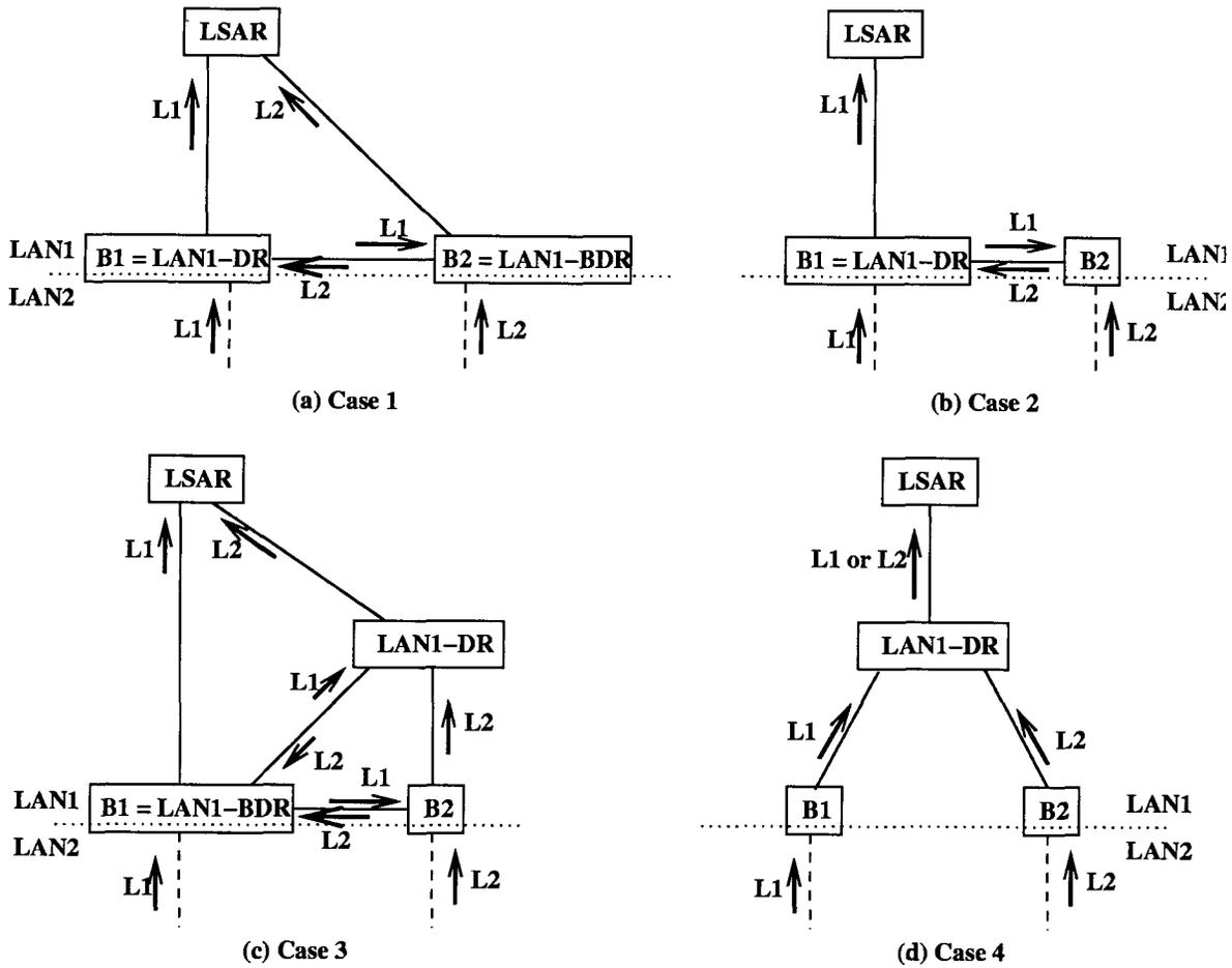
Fig. 12. Control-plane diagram for LAN 1 under different roles played by the *B*-pair routers. The figure also shows how different copies of LSA *L* can arrive at the LSAR via the *B*-pair routers. *L1* and *L2* are copies of LSA *L*.
